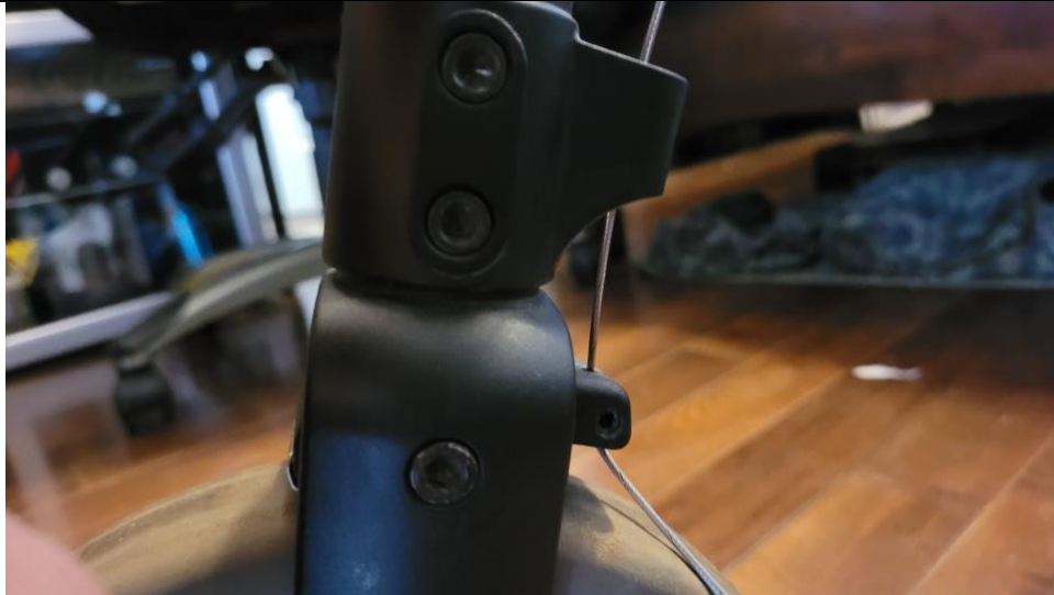
Figure 6.17: Loosening the tensioning screw
