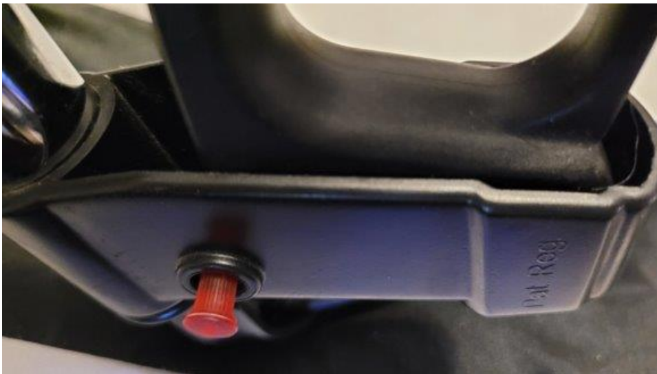
Figure 4.1.1 Rotary Encoder Friction Lock Pin
