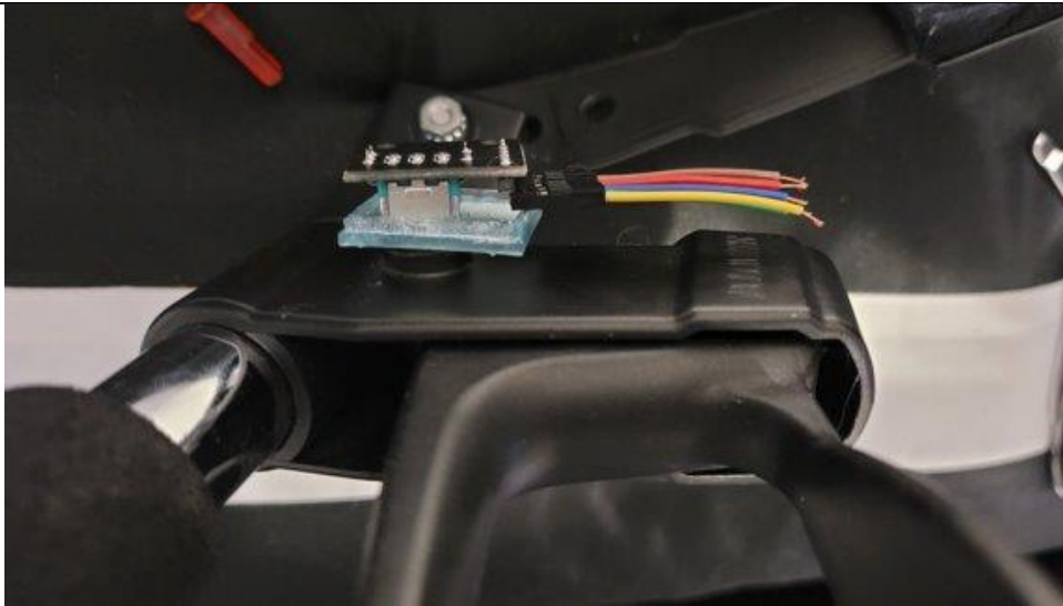
Figure 4.1.2 Rotary Encoder Mounted on Side Handle
