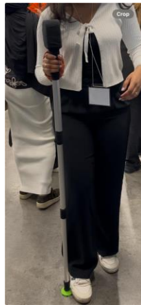
Figure 13: Person stepping on tip and twisting out the locking mechanism.
