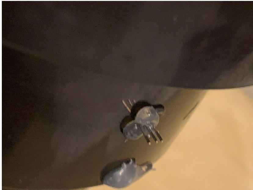
Figure 16 - Temperature Sensor with protruding pins
