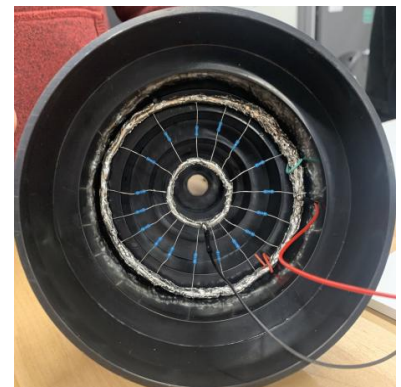
Figure 15 - Resistor ring and housing
