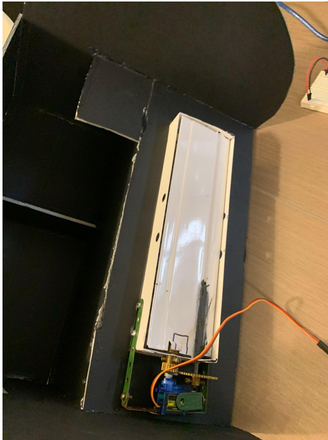
Figure 10 - Servo control for register
