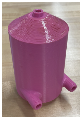
Figure 18 - 3D printed sump pump used in final design
