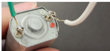
Figure 7: Soldered connection between the jumper cables and the prongs of the DC motor.
