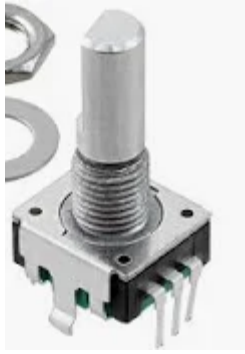
Figure 6: Rotary encoder.
