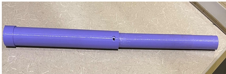
Figure 8 - Prototype 2, Telescoping Tubes
