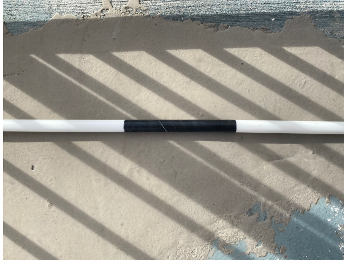
Figure 1: Physical prototype of the PVC handlebar with the rubber coated middle section
