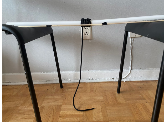
Figure 3: Testing installation to measure the deflection under weight of each bar
