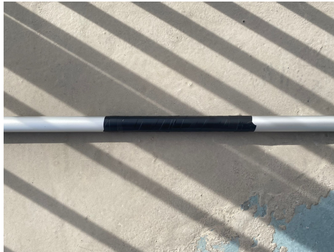
Figure 2: Physical prototype of the metal alloy handlebar with the rubber coated middle section
