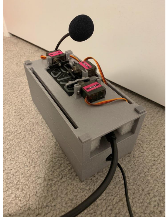
Figure 1. CAD schematic (on left) and photo (on right) of our prototype. The bottom layer houses the electronics, the middle layer houses the remote, and the top layer houses the servo motors.
