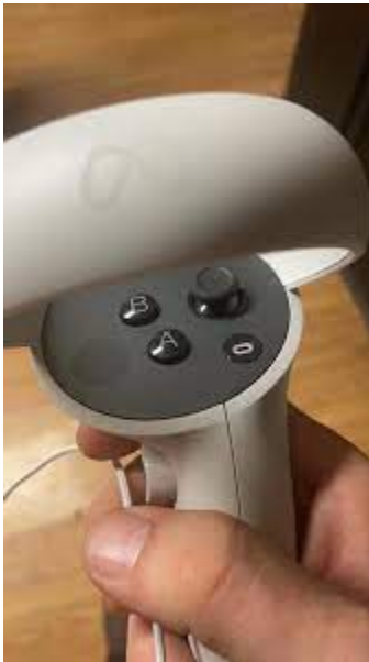
Figure 3.5.1 -The button with the oval shape on it in the bottom right can be used to exit the system.
